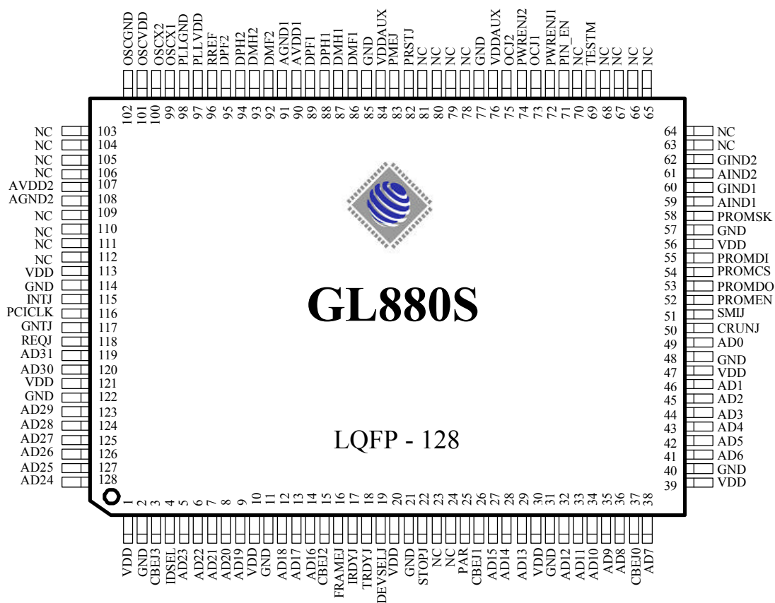
Figure 3.1 - Pinout Diagram
