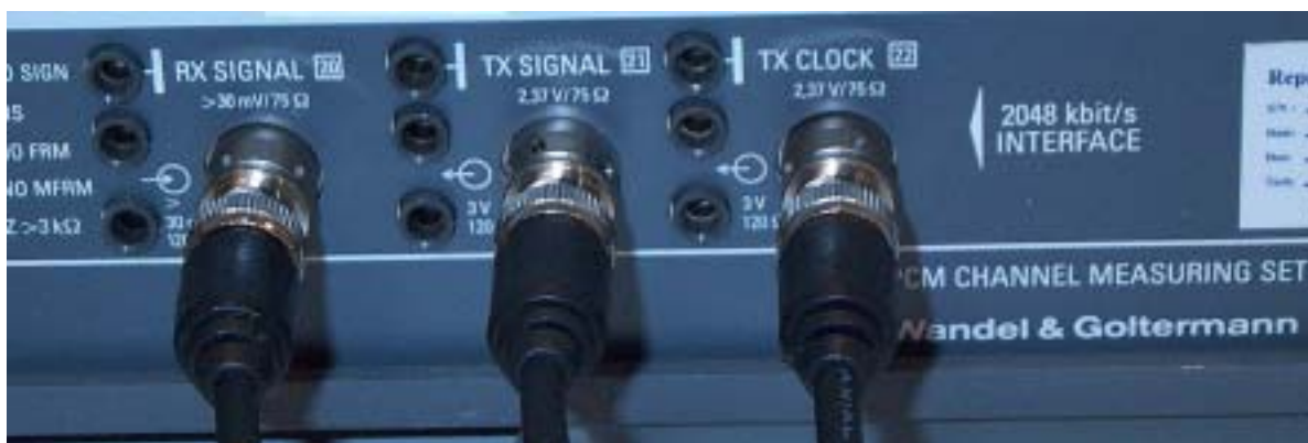
Figure 2. W&G PCM-4 Signal and Clock Connections
