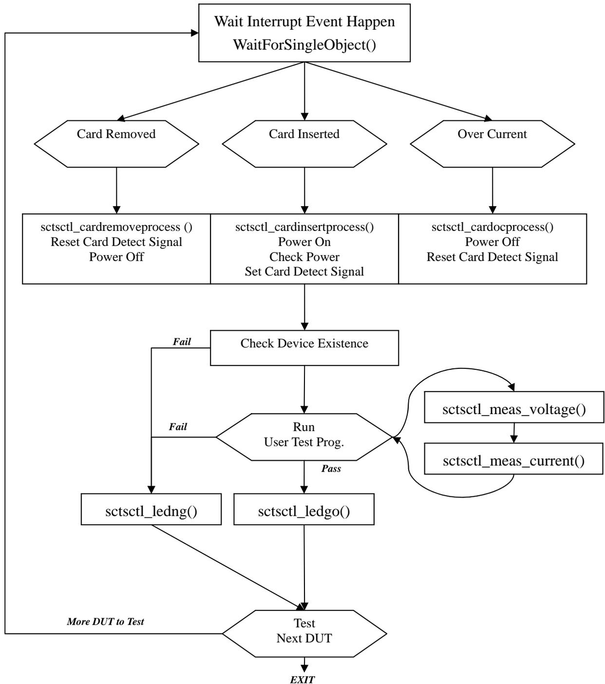
Fig. 2: Operation/Test Flow
